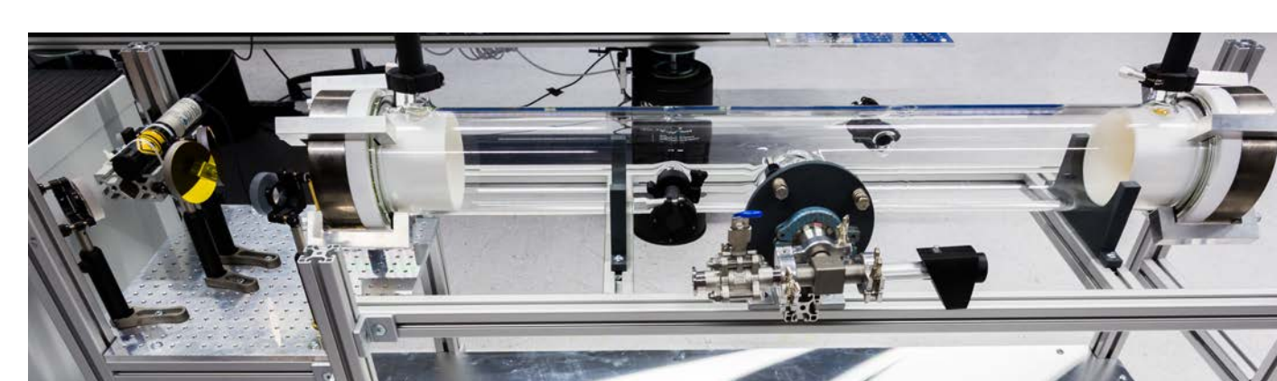
Figure 7: New built multipass spectrometer at Kassel
